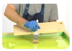
As you lower the planks tilt them on the long edge and lower slowly with a slight rocking motion until the plank is sitting on the resin. This will help to prevent air pockets being trapped on the underside of the planks.
